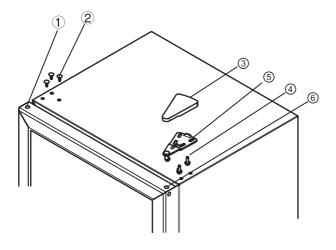
• Open the door of the Beverage Chiller cabinet so the seal doesn't hold it in place and carefully detach the glass door by sliding it upwards. Place it aside on a soft surface.
