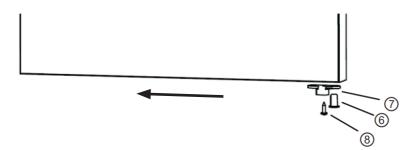
Using two people, lay the unit down on its back. Dismantle the adjustable foot (11), positioning bolts
