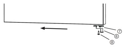
Using two people, lay the unit down on its back. Dismantle the adjustable foot (11), positioning bolts
