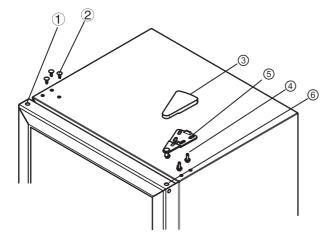
• Open the door of the Beverage Chiller cabinet so the seal doesn't hold it in place and carefully detach the glass door by sliding it upwards. Place it aside on a soft surface.
